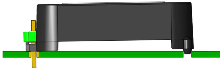
Figure 16: Mini Package with interference-fit of PCB-locating features
