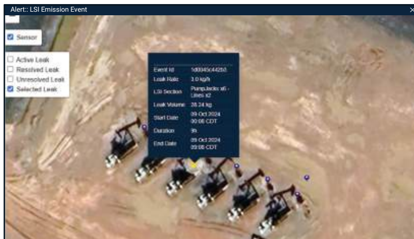
Emission details specifying location, volume, and duration of leak
