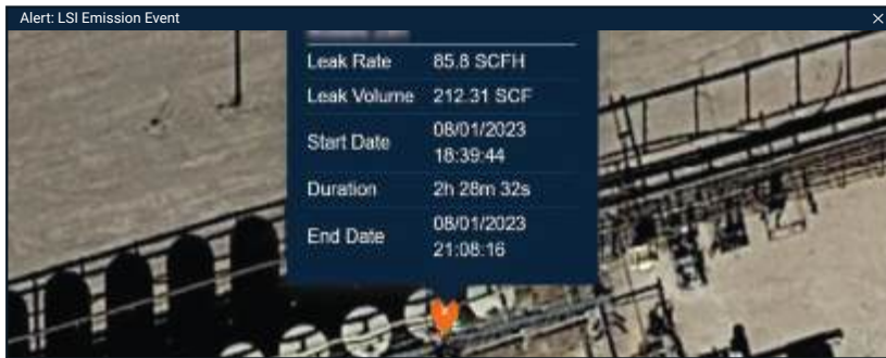
Emission details on MethaneTrack™ platform specifying location and volume of leak
