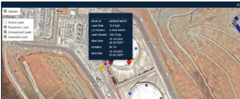
Emission details on MethaneTrack™ specifying location, volume, and duration of leak
