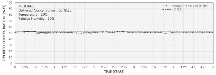
Average concentration reported to repeated exposures of 50 %LEL methane vs. time. Between exposures, all sensors were operated without airflow in ambient air. During exposures, all sensors were placed in an environmental chamber set at standard conditions (20  $^{\circ}$ C, 50 %RH) where gas was delivered from a cylinder. Accuracy remains within  $\pm 3$  %LEL over 5 years.
