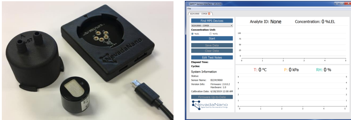
Figure 1: On the left, the “Evaluation Kit” hardware; on the right, the “MPS Flammable Gas Sensor interface” application.
