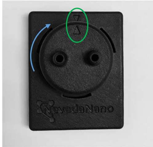
Figure 2 – Proper gas mask attachment is achieved when the arrow points align and the barbs are in the horizontal position.
