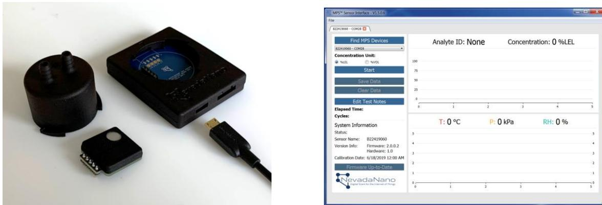
Figure 1: On the left, the “Evaluation Kit” hardware; on the right, the “MPS A2L Refrigerant Gas Sensor interface” application.
