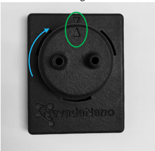
Figure 3 – Proper gas mask attachment is achieved when the arrow points align and the barbs are in the horizontal position.
